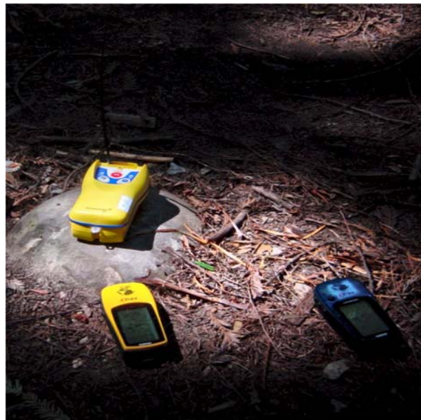
Fastfind Plus PLB on the ground under cover of redwood trees. The satellite coverage monitored on the two Garmin receivers varied between 1 and 3 satellites throughout the test.
