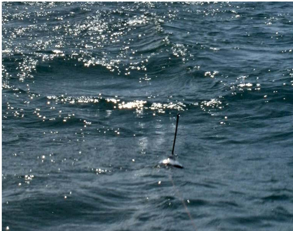
G4 EPIRB floating at sea restrained on its lanyard
