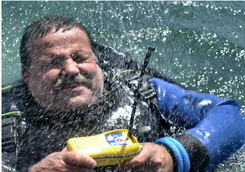
Swimmer and Fastfind Plus PLB under simulated heavy rain
