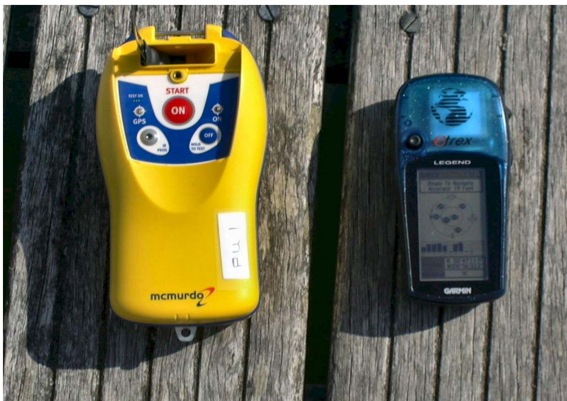
Activation of a Fastfind Plus PLB on a pontoon at Sparkes Marina. There are 7 satellites clearly visible on the Garmin eTrex.
