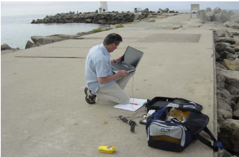
Baseline Scenario Alpha, concrete jetty at Santa Cruz yacht harbour Setting up the beacon message logging equipment prior to activation of a Fastfind Plus PLB
