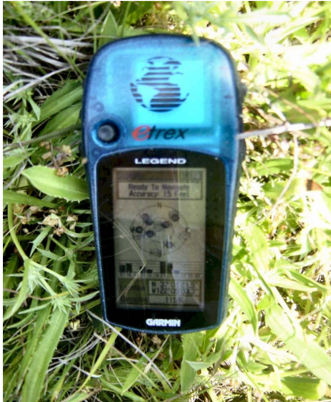
Five strong satellite signals displayed on Garmin eTrex Legend (7 visible).
