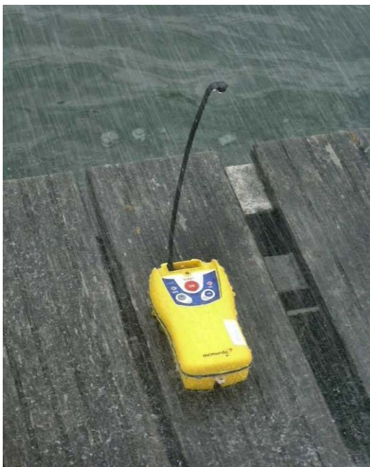
Fastfind Plus PLB under heavy spray
