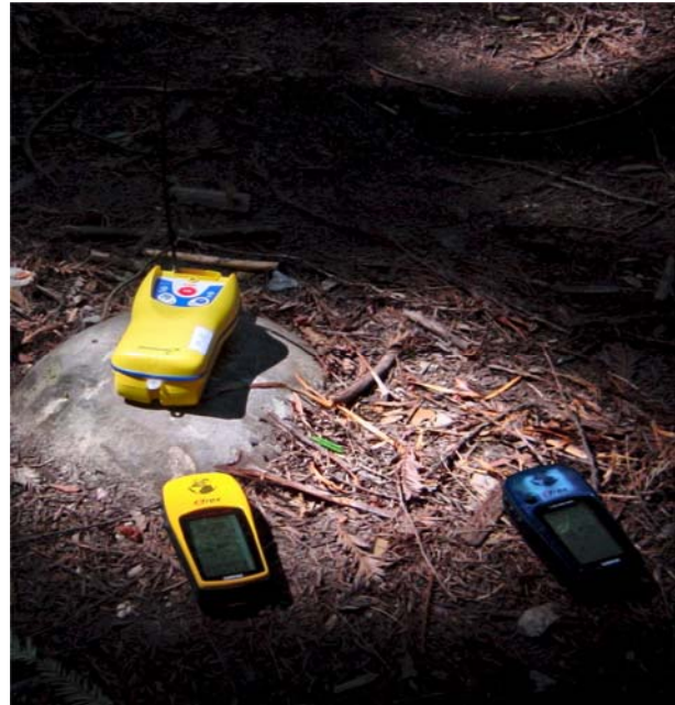
Fastfind Plus PLB on the ground under cover of redwood trees. The satellite coverage monitored on the two Garmin receivers varied between 1 and 3 satellites throughout the test.
