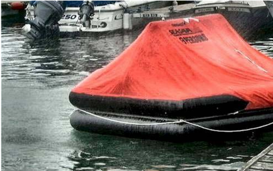
Three hoses being played on the closed liferaft to simulate heavy rain
